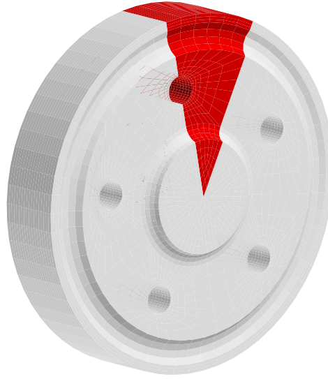
Figure II.3 : Free turbine disk geometry
