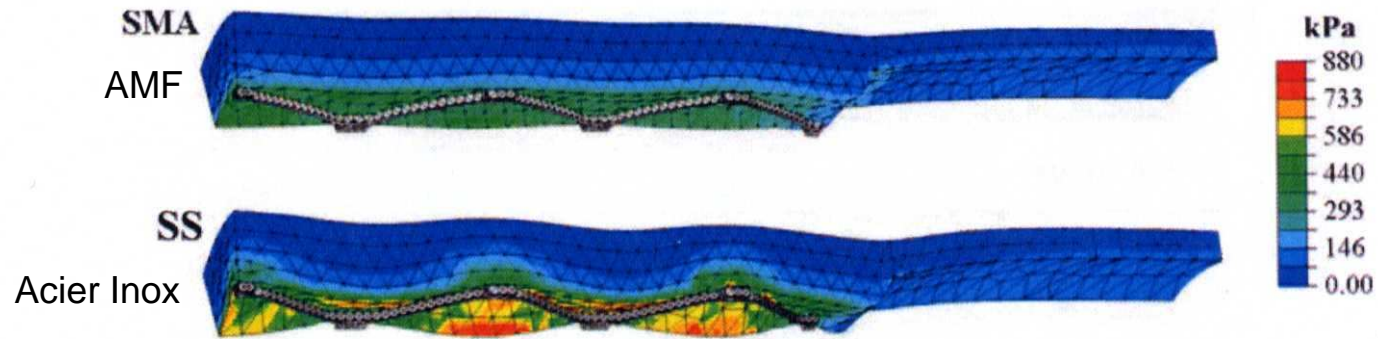
Fig. 10. Von Mises stress maps with an expanded internal vessel diameter of 3.2 mm for the self-expandable SMA stent (top) and the SS stent (bottom)
