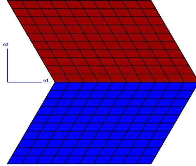
Figure 2: Tension of a twin laminate with periodicity conditions. The horizontal direction  $x$  is the tensile direction. The vertical direction  $z$  is the normal to the twin boundary. The red and blue colors denote the A and B crystals. Deformation is strongly magnified compared to reality.
