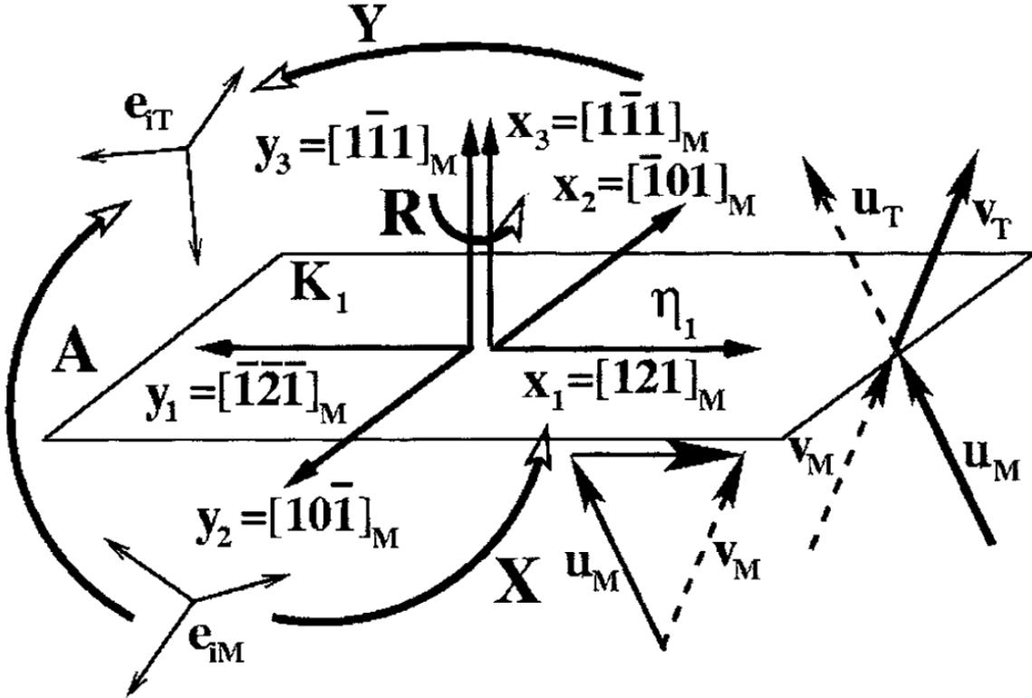
Figure 1: Characteristics of the twin boundary and orientations of crystals, after [1]. We call  $A$  the crystal below the plane and  $B$  the twin crystal above the plane. These names are not indicated on the drawing (the letter  $A$  here has a different meaning).
