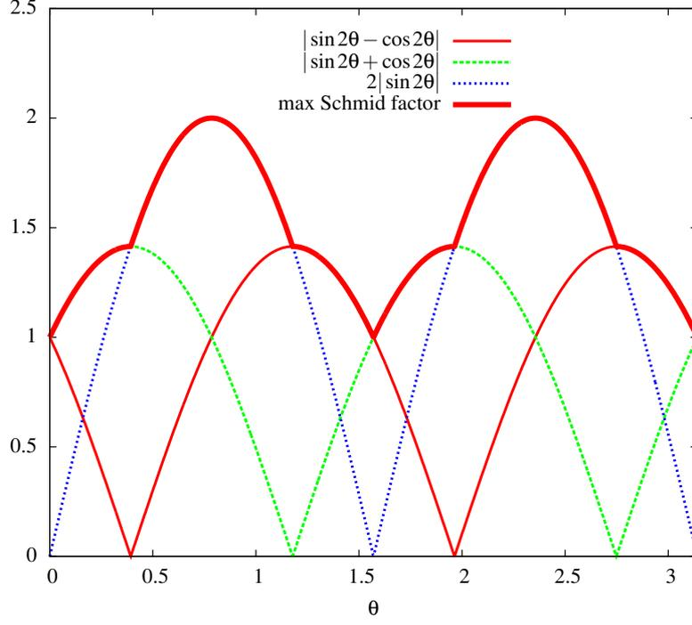
Figure 2: Schmid factors for the simple shear of a single crystal as a function of the  $\theta$  orientation angle.
