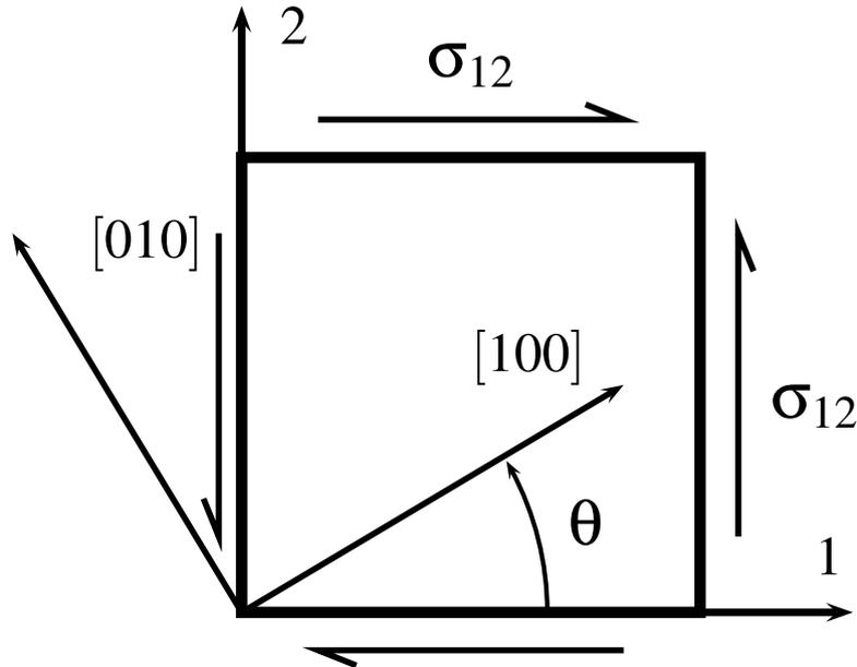
Figure 1: Orientation of a single crystal with respect to the coordinate system of the loading.
