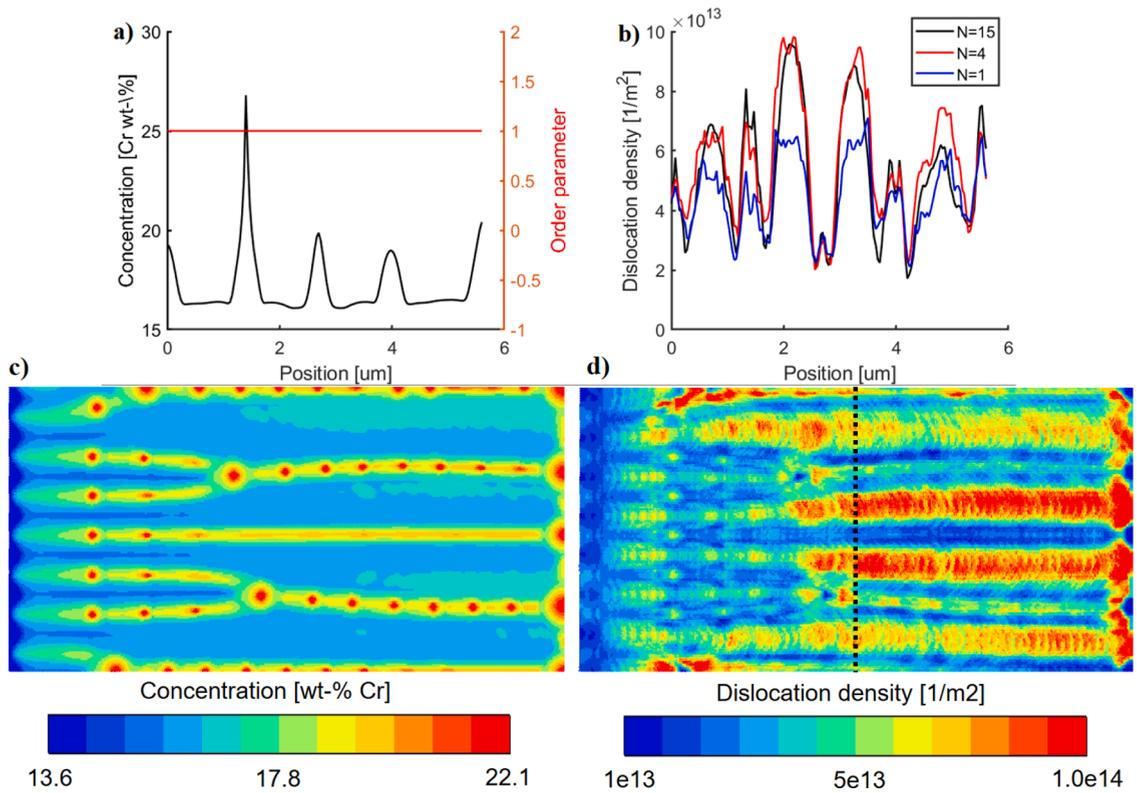
Fig. A.8. Sensitivity analysis on parameter  $N$ . a) Concentration and order parameter from PF, b) dislocation density over a line, c) concentration map, d) dislocation density map. Contours c) and d) are produced using  $N = 1.0$ .
