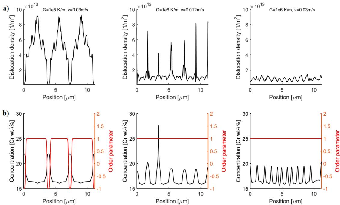
**Fig. 6.** Line profiles in the middle of the simulation box, in vertical direction, for the different cases, a) dislocation density with MPC boundary conditions, b) concentration (black) and order parameter (red) from PF simulations. (For interpretation of the references to colour in this figure legend, the reader is referred to the web version of this article.)
