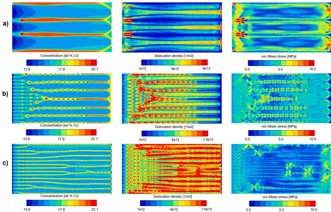
**Fig. 5.** Concentration of chromium, dislocation densities, and von Mises stress contours for a)  $G = 10^5$  K/m and  $V = 0.03$  m/s, b)  $G = 10^6$  K/m and  $V = 0.012$  m/s, c)  $G = 10^6$  K/m and  $V = 0.03$  m/s.
