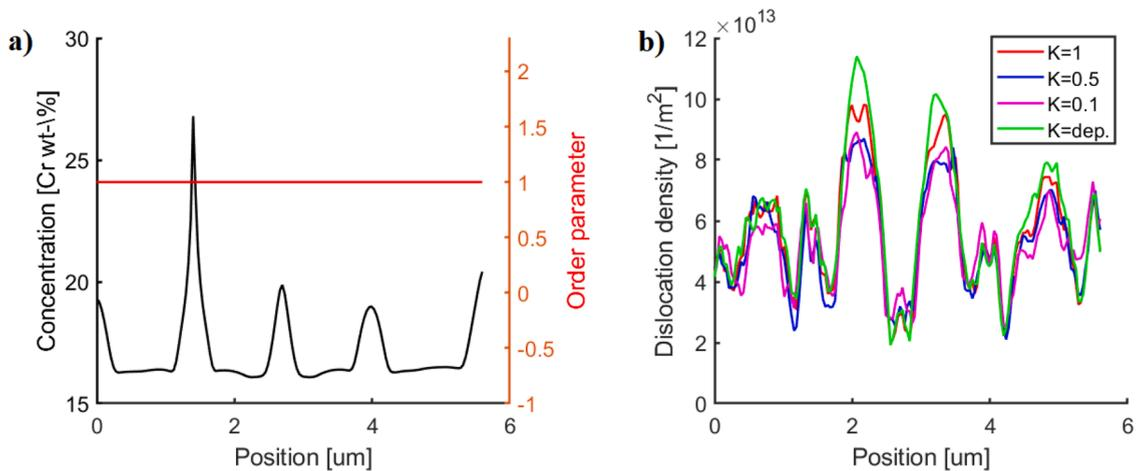
Fig. A.9. Sensitivity analysis on parameter  $K$ . a) Concentration and order parameter from PF and b) dislocation density over a line. Value for  $N$  is 4.0 except for the case where  $K$  is dependent on concentration  $C$ .
