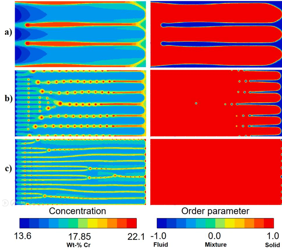
Fig. 4. Solute segregation and order parameter mappings at the end of simulation for a)  $G = 10^5$  K/m and  $V = 0.03$  m/s ( $Q = 3 \times 10^3$  K/s), b)  $G = 10^6$  K/m and  $V = 0.012$  m/s ( $Q = 12 \times 10^3$  K/s), c)  $G = 10^6$  K/m and  $V = 0.03$  m/s ( $Q = 30 \times 10^3$  K/s).
