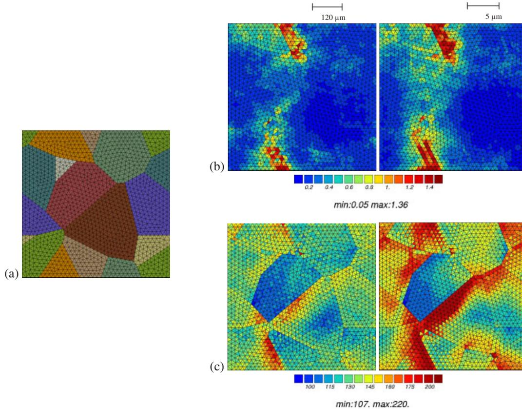
**Fig. 1** Finite element simulations of the shear deformation of the 2D aggregates of figure 1 with different grain sizes: (a) mesh of the grains (b) norm of the plastic curvature tensor (unit  $mm^{-1}$ ); (c) Von Mises equivalent stress fields (unit MPa). The geometry of the grains is the same for both computations but the absolute size of the aggregates differ. Geometrical and kinematical periodicity conditions are imposed.
