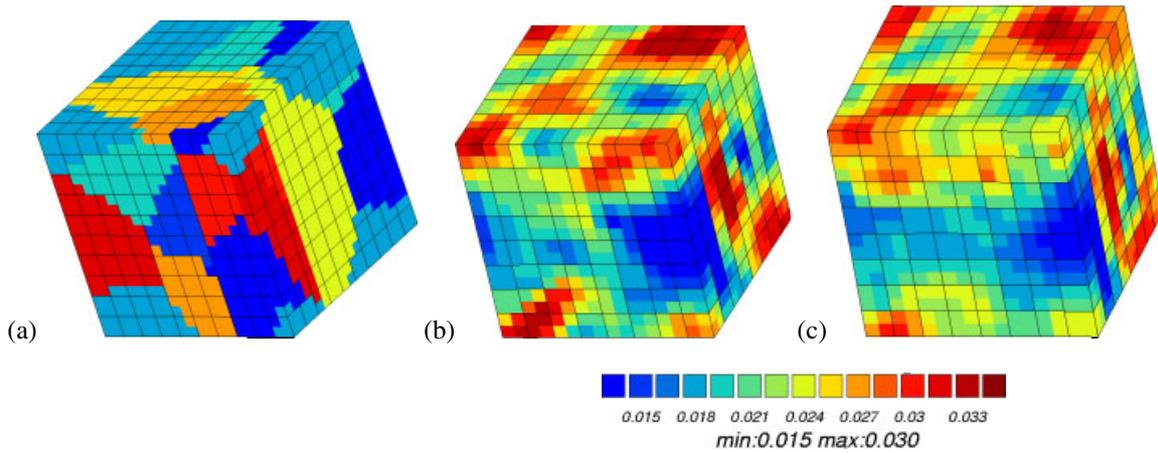
**Fig. 2** Finite element simulations of the tensile test of tridimensional aggregates containing 10 grains : (a) mesh of the grains (b) and (c) maps of the equivalent plastic strain (unit MPa) after 0.075% mean strain and for a grain size respectively equal to 120 μm and 5 μm. Geometrically and kinematically boundary conditions are imposed.
