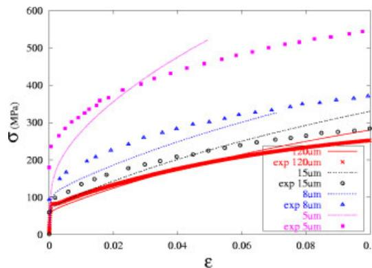
**Fig. 3** grain size effect in ferritic steel : experimental and simulated results
