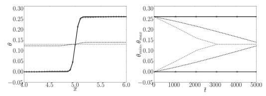
**Fig. 3.** Profiles of  $\theta$  at  $\bar{t}=5000$  (left) and evolution of  $\theta$  over time (right). Solid line: Cosserat coupling modulus is active (d)  $\mu_c/f_0=1000$ . In the other cases, it is not active. Gray line with stars (a):  $\overline{\mu}_P=1000$ ,  $\overline{\tau}_\theta=1000$ . Dashed-dotted line (b):  $\overline{\mu}_P=5$ ,  $\overline{\tau}_\theta=1000$ . Dashed line (c):  $\overline{\mu}_P=1000$ ,  $\overline{\tau}_\theta=1000$ .
