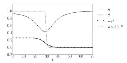
**Fig. 10.** Evolution in time of  $\eta$  and  $\theta$  together with  $\rho$  at a fixed point swept by the moving GB.
