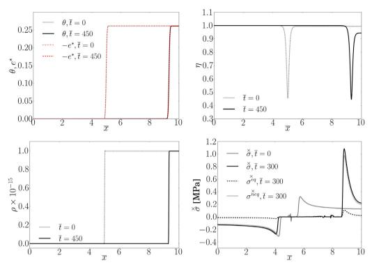
Fig. 7. Tracking of the moving grain boundary. Top left and right shows the profiles of  $\theta$  and  $\eta$ , respectively, at  $\bar{t}=0$  and  $\bar{t}=450$ . Bottom left shows  $\rho$  at  $\bar{t}=0$  and  $\bar{t}=450$ .
