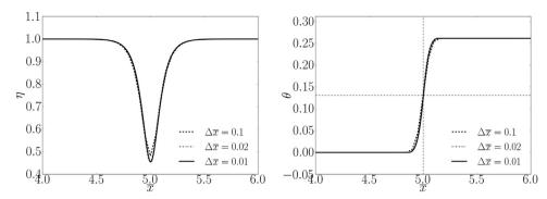
**Fig. 2.** Grain boundary profiles of  $\eta$  (left) and  $\theta$  (right) at equilibrium for the KWC model. Solid lines: 2000 elements ( $\Delta \bar{x} = 0.01$ ); dashed-dotted lines: 1000 elements ( $\Delta \bar{x} = 0.02$ ) and dashed lines: 200 elements ( $\Delta \bar{x} = 0.1$ ).
