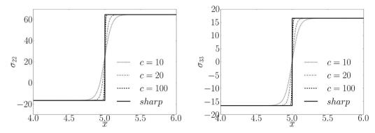
Fig. C1. Analytically resolved stress profiles for pure shear loading and anisotropic elasticity. The solid line is the sharp interface solution and the other lines represent tanh formats of the orientation with increasingly high prefactor.
