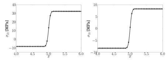
**Fig. 6.** Calculated stress profiles for simple shear loading and anisotropic elasticity. Solid lines show the result from finite element calculations and dashed lines with markers show the analytic solution. Left:  $\sigma_{22}^s$  and right:  $\sigma_{33}^s$  with 1000 finite elements.
