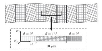
Fig. 1. A microstructure made of periodically replicated bicrystal layers is represented by a periodic geometry used for simulations. The misorientation between the layers is 15°.
