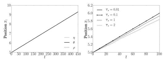
**Fig. 8.** Position of the grain boundary center over time (left) for the respective profiles of  $\eta$ ,  $\theta$  and  $\rho$ . The influence of the parameter  $\overline{\tau}_*$  on the velocity of the grain boundary migration is also shown (right). Note that the solid line ( $\overline{\tau}_* = 0.01$ ) and the solid line with star markers ( $\overline{\tau}_* = 0.1$ ) coincide.
