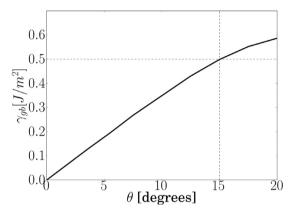
Fig. B.12. Grain boundary energies for misorientaions up to  $20^{\circ}$  and  $f_0 = 8.2$  MPa, calibrated to an approximate grain boundary energy of  $0.5 \,\mathrm{J/m^2}$  at  $15^{\circ}$  misorientation.
