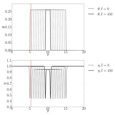
**Fig. 9.** Evolution in time of  $\theta$  and  $\eta$  at discrete time steps  $\Delta \bar{t} = 50$ . The dislocation free grain grows and will eventually annihilate the grain of high stored dislocation density. The red line shows the position of the fixed node where results are extracted over time in Fig. 10. (For interpretation of the references to color in this figure legend, the reader is referred to the web version of this article.)
