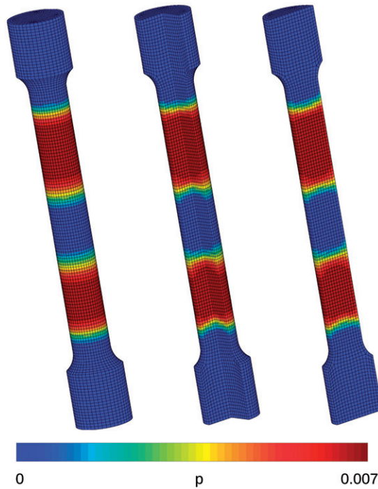
Figure 19. Evolution of cumulative plastic strain at the strain rate 10^{-3} \text{ s}^{-1} with the boundary conditions of Figure 18a. View of the outer surface (left), 3/4 of the specimen (middle), and one half of the specimen (right).
