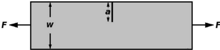
Figure 12. Illustration of a SEN geometry corresponding to the Equation (54), where B is the specimen thickness.
