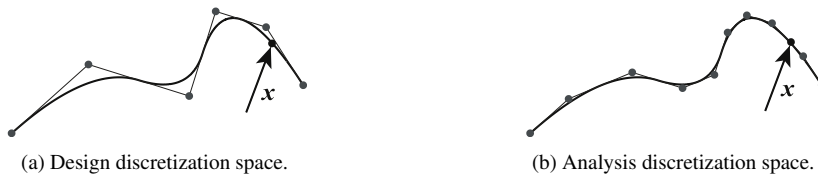
Fig. 6. Two levels NURBS discretizations: (a) Coarse discretization for design, (b) Refined discretization for analysis.
