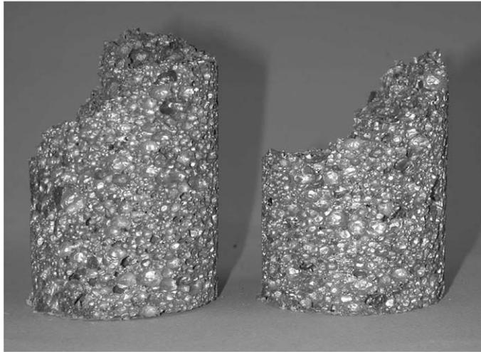
Fig. 10. (a) Stress–Strain curve for a specimen in torsion. (b) Corresponding fracture surface of the specimen (specimen diameter: 65 mm).
