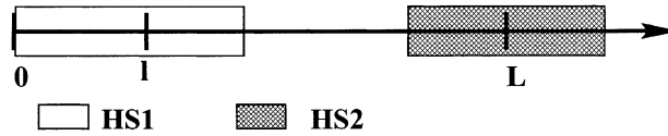
Fig. 1. Range of possible variation of intrinsic length l_c with respect to the characteristic lengths of the problem for the homogenization problems considered in this work.
