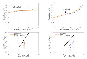
The model is able to predict baseline growth and OL transient behavior for both materials within a factor of 2 in terms of number of cycles (equivalent crack length).
