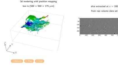
ICF12, Ottawa - 3D monitoring and modelling of small corner cracks in Al alloys
